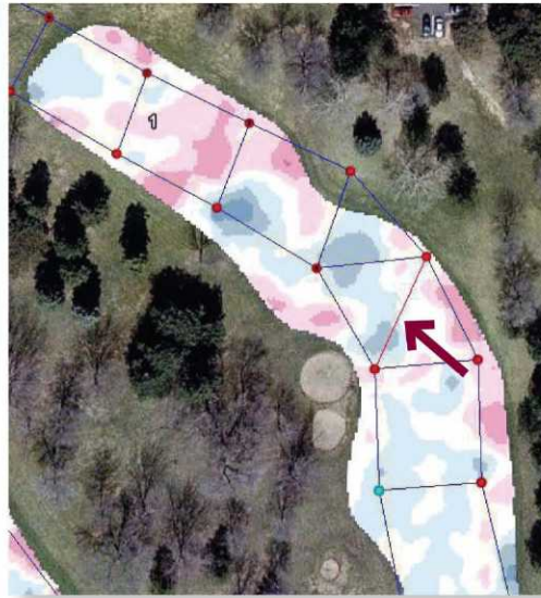
Figure 3. Assessment of distance between adjacent irrigation heads on fairway 1. Any heads that are more than 92.6 feet apart (which is 1 standard deviation above the mean spacing for the fairway) are red-flagged for closer observation as to whether they are contributing to soil volumetric water content issues. 1 SD would identify distances between heads that are within the highest 16% of all spacings on a course. However, on this fairway, even the mean distance between irrigation heads is large, based on the heads, nozzles and operational pressure used. For this fairway, the mean distance is 85.0 feet (25.9 meters); the minimum distance is 60 feet (18.2 meters); the maximum distance is 116.9 feet (35.6 meters); the standard deviation is 7.6 feet (2.3 meters); and the coefficient of variability is 9%.
